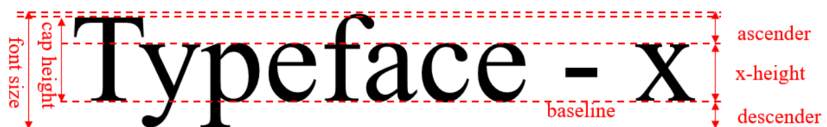
Figure 1: Explanation of font size and x-height based on a figure (presented in German) in a publication of the Deutscher Blinden- und Sehbehindertenverband e.V. (DBSV) [63].
