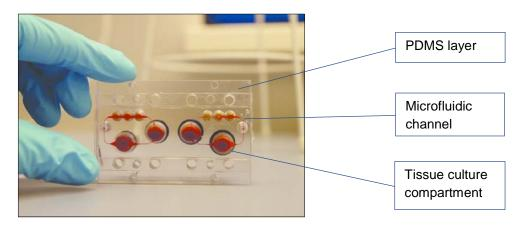
Figure 5: Multi-organ-chip with PDMS layer, Source: [86]
