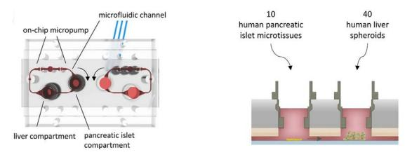
Figure 6: Two-organ-MPS (liver-islet-chip). Structure of liver-islet-chip device (left), tissue-loading scheme of organ co-culture (right), Source: [87]
