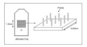
Figure 13: Illustration of an Affymetrix Gene Chip, Source: [99]
