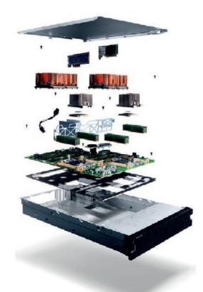
Power System AC922 internal components
